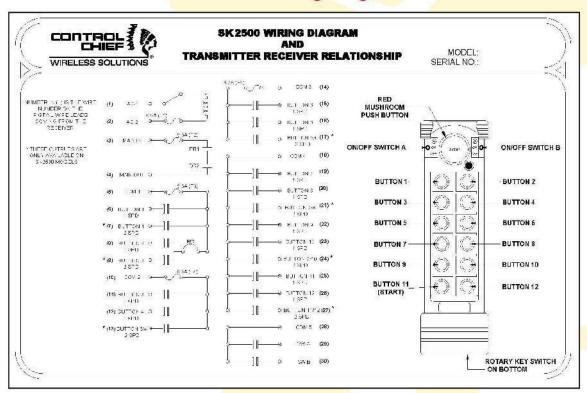
Wiring diagrams for reference only - not for installation
