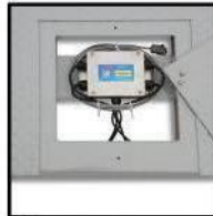
SS on-board junction box
