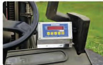
Model CSW-10AT-LFT Indicator viewed from inside Lift Truck
